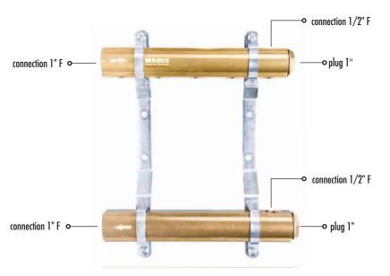
Brass manifold **CM** is responsible for distribution and regulation of the heating medium. The manifold allows connecting different circuits and installation zones, increasing the efficiency of the heating system. It contains two C-profile beams connected with two steel holders, connections for air vents and connections for supply and return of the system.
